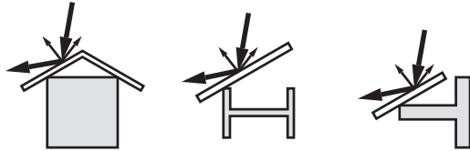
Fig. 14: Cover flat, large-area profiles with deflectors
