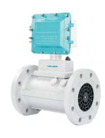
Gas turbine flow meter take into account the compressibility of gases, and the correlation between volume, temperature and pressure of the medium. To convert Process Work Condition medium to Standard Condition, temperature and pressure sensors are added to track temperature and pressure changes of the measuring medium.
