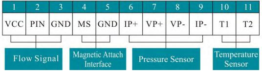
1)The flow meter can receive processed signals and can supply power to the signal processing board. The wiring is as followings:
