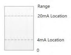
As shown in the figure, when the liquid level is lower than 4mA Location, the main interface displays the liquids level as 0;
