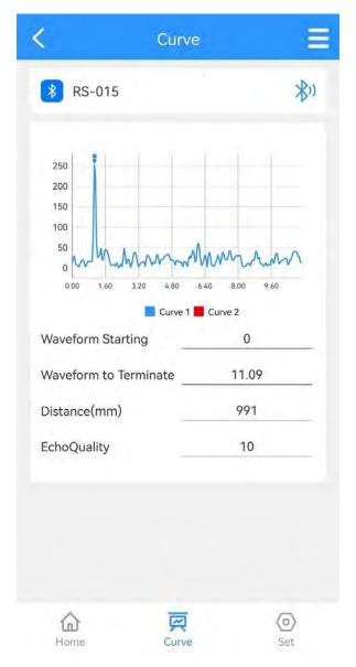
Waveform Starting: The starting position of the waveform
