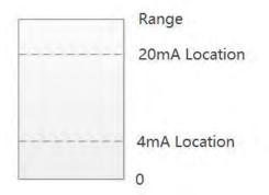
As shown in the figure, when the liquid level is lower than 4mA Location, the main interface displays the liquids level as 0;
