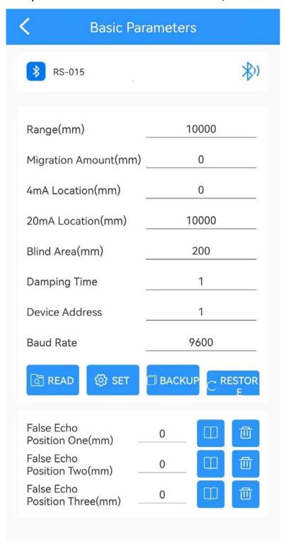
Set the "Range" according to the working conditions and directly click the number input box behind to modify it. The rest of the parameters are modified in the same way.
