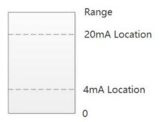
As shown in the figure, when the liquid level is lower than 4mA Location, the main interface displays the liquids level as 0; when the liquid level is higher than the 20mA location, the main interface displays the liquid level value as the value of 20mA location.
