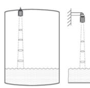
Vertical installation without aiming of the antenna
