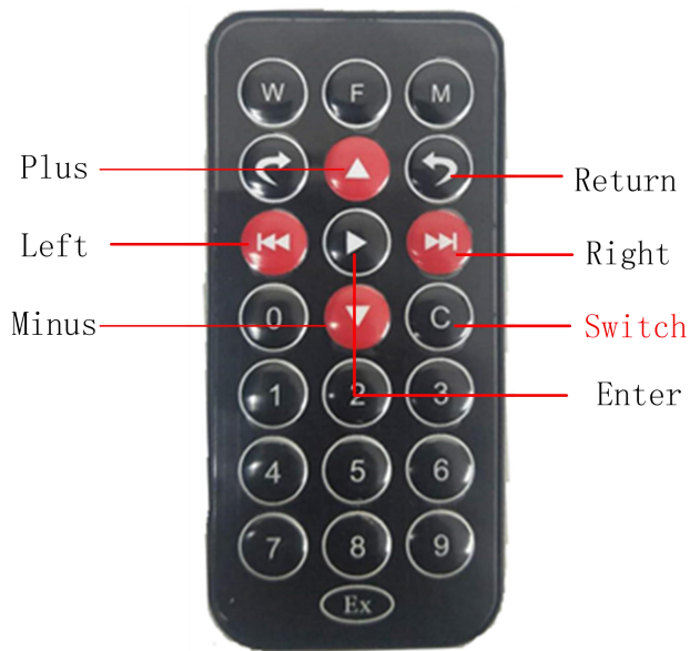
Fig3.1.3 Definition and operation of infrared remote control keys
