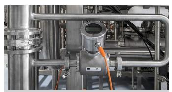
With the FMQ flow meter, too, a single cable provides power supply and data exchange in both directions. Thanks to IO-Link, the sensor can be monitored via the Internet and actively programmed and parameterized.
