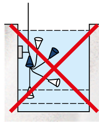
Image 6. Avoid fixing the float such that a sharp corner can cause kinks or wear to the cable.
