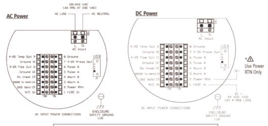
\*⚠ This is not a Loop powered device. ◆ Do not apply power to 4-20 mA Loops. ◆ 4-20 mA Loops are active (non-isolated)
