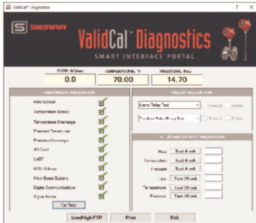
Figure 1. SIP ValidCal Diagnostic Test Results showing all systems are OK
