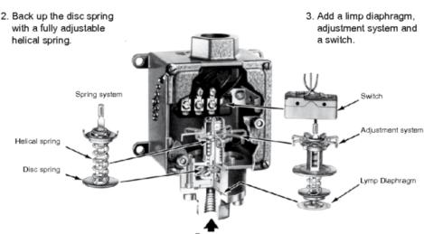
By replacing the elastic creep deflection of conventional pressure switch sensors with the negative spring rate of a disc spring combination pressure switches have now become binary like computers. This revolutionary design has been proven to be so reliable that on jet aircraft, for instance, it has been the only design acceptable for many decades.
